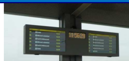
Pic. 19: Double departure LCD panel (2x21") with a clock – the ELP A821EH type.
